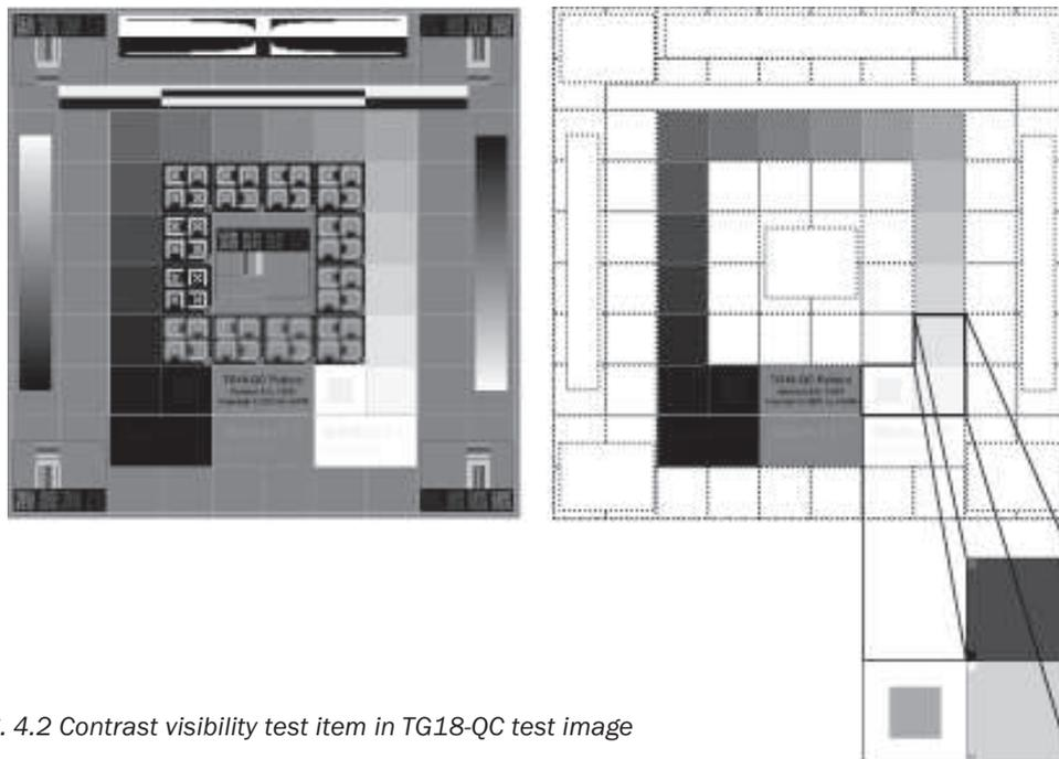
Fig. 4.2 Contrast visibility test item in TG18-QC test image
