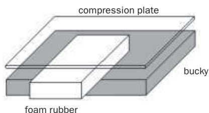
Fig. 2.5 Compression plate alignment measurement, symmetrical load
